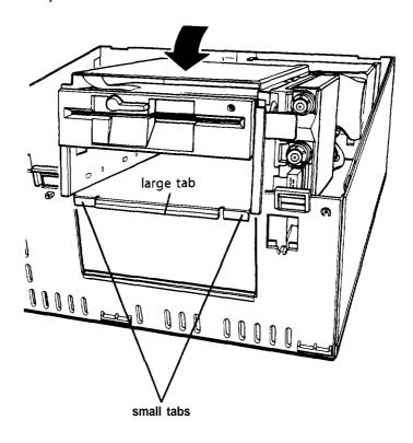
Guide the tabs on the front of the subassembly over the opening in the front of the computer so that the two small tabs sit behind the opening and the large tab with the curved lip sits over the front. If necessary, press on the large tab until the subassembly snaps into place.
